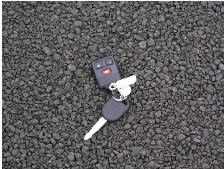
Figure PT-2.4: Washed aggregate base with keys for scale.
