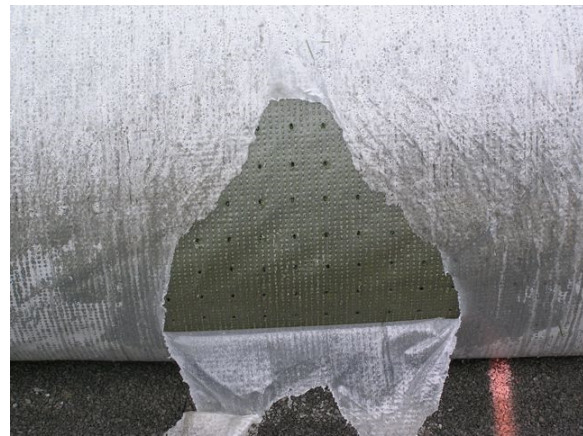
Figure PT-2.6: Underside of permeable artificial turf, showing drainage holes.
